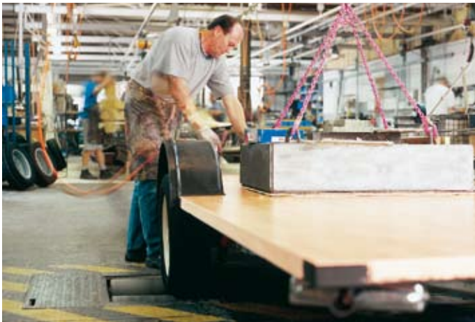
Basic operation: fitting HICOTEC® TP heating film underneath the PVC floor covering on the chassis plate.
